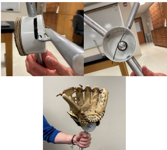
Figure 1: Clutch Catch assistive device. Clockwise from top left, slider view, interior view, device in glove.
