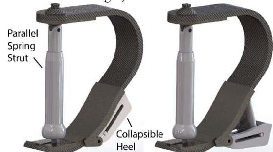
Figure 1: Rendering of the prosthetic prototype with the Parallel Spring Strut and the Collapsible Heel (collapsed on the left, deployed on the right).
